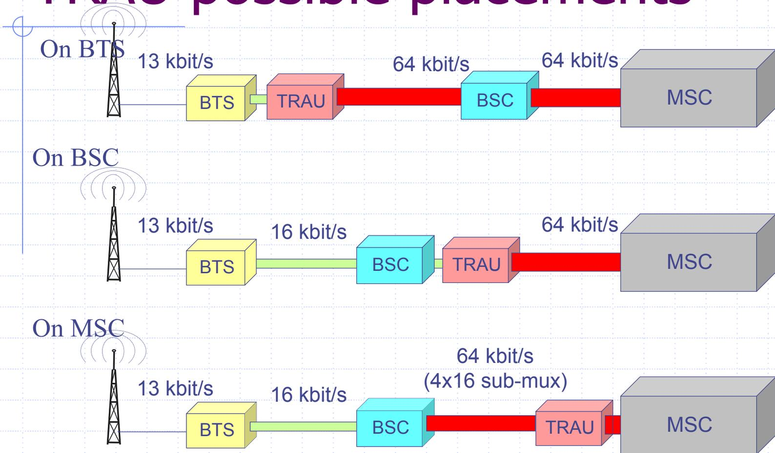
*Why 16 kbps instead of 13? Inband signalling needed for BTS control of TRAU (TRAU needs to receive synchro & decoding information from BTS)*
