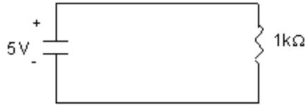
Figure 1. Simple resistor circuit.
