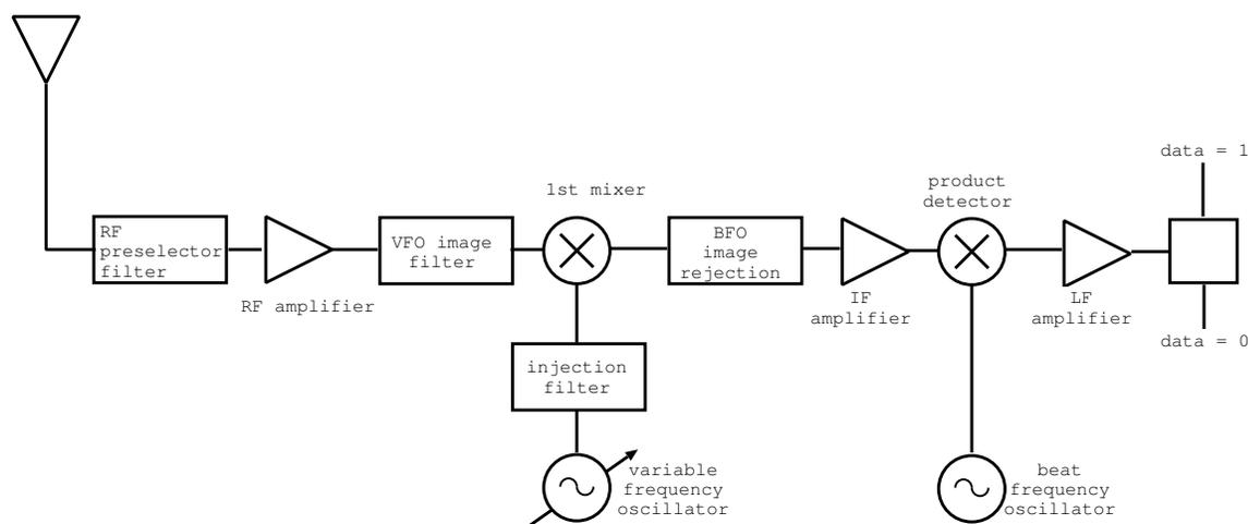
Figure 1: Superheterodyne receiver structure.
