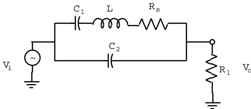
Figure 1: Resonance Circuit.
