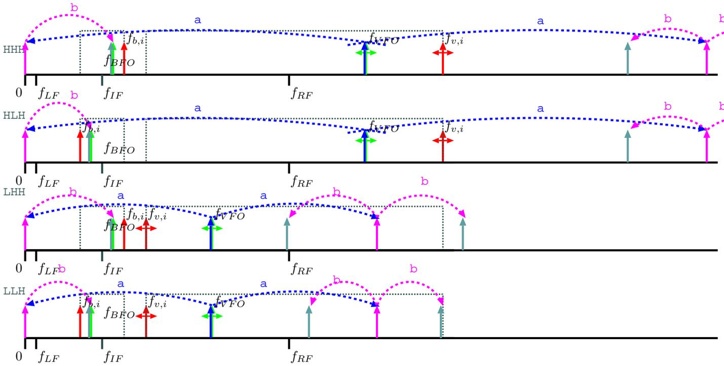
Figure 5: Four possible solutions to part 1c, when considering spurious components at  $f_{VFO}$ . Frequency axis not to scale, and the translation of each spurious signal is indicated by colored arcs, with the translation amount as the arc label, as in Figure 2. Label  $a$  represents a translation by an amount  $f_{VFO}$ , label  $b$  denotes a translation by an amount  $f_{BFO}$ .
