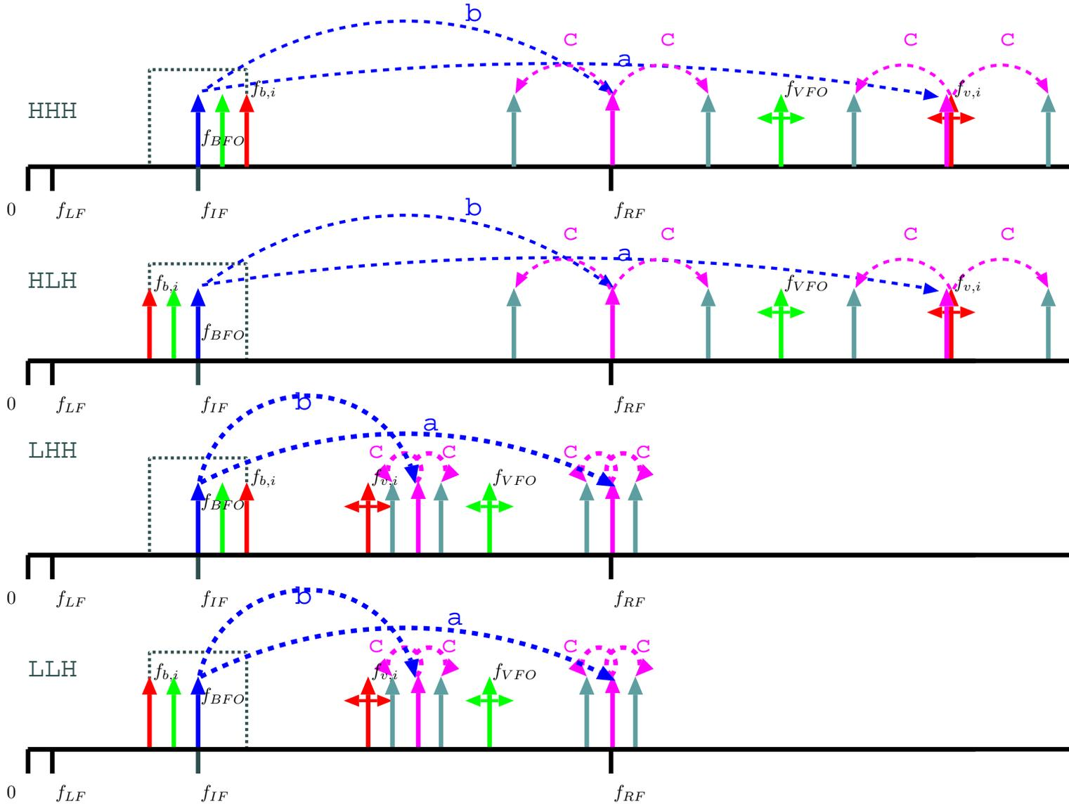
Figure 4: Four possible solutions to part 1c, when considering spurious components at  $f_{IF}$ . Frequency axis not to scale, and the translation of each spurious signal is indicated by colored arcs, with the translation amount as the arc label, as in Figure 2. Label *a* represents a translation by an amount  $f_{VFO}$ , label *b* denotes a translation by an amount  $|f_{IF} - f_{VFO}|$ , label *c* denotes a translation by an amount  $f_{BFO}$ .
