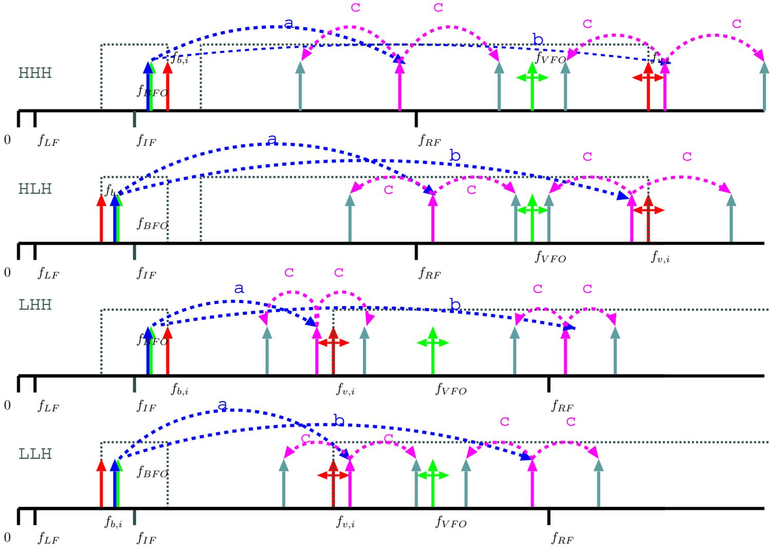
Figure 6: Four possible solutions to part 1c, when considering spurious components at  $f_{BFO}$ . Frequency axis not to scale, and the translation of each spurious signal is indicated by colored arcs, with the translation amount as the arc label, as in Figure 2. Label  $a$  represents a translation by an amount  $f_{VFO} - f_{BFO}$ , label  $b$  denotes a translation by an amount  $f_{VFO}$ , and label  $c$  denotes a translation by an amount  $f_{BFO}$ .
