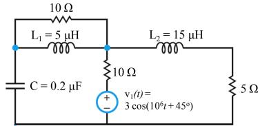
2B) For this circuit, apply the **Node-voltage method** in phasor domain to give two systems of equations and two unknowns node voltages **V1** and **V2**. Write these, simplify and put in **matrix form** below. Place a box around your final answer to make it easy for a grader to find. YOU DO NOT HAVE TO SOLVE V1 and V2. **(8 Points)**
