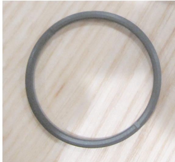
Retaining Ring (note slots)
