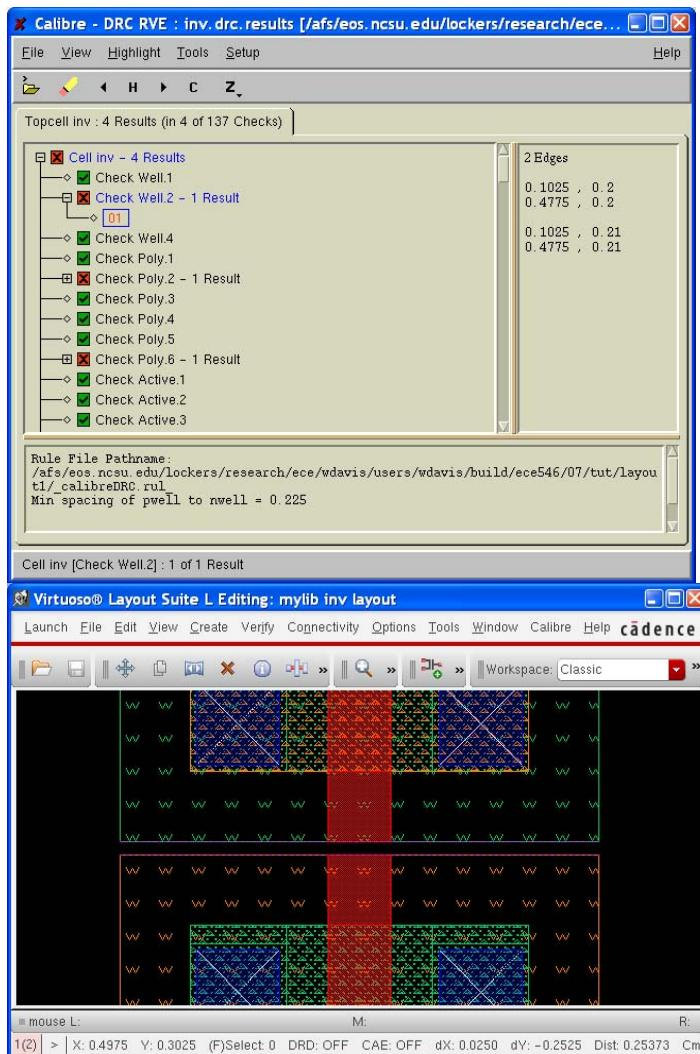
In this particular case, the transistor wells are too close together. Fix this error by moving up the pmos. It's good practice to space the NMOS and PMOS transistors by the smallest amount allowed in order to make the layout as dense as possible. You can draw temporary rulers by hitting "k" and dragging a ruler. You can clear the rulers by hitting "Shift-K". These rulers can help you to draw dense layout much faster than you would by constantly running DRC.
