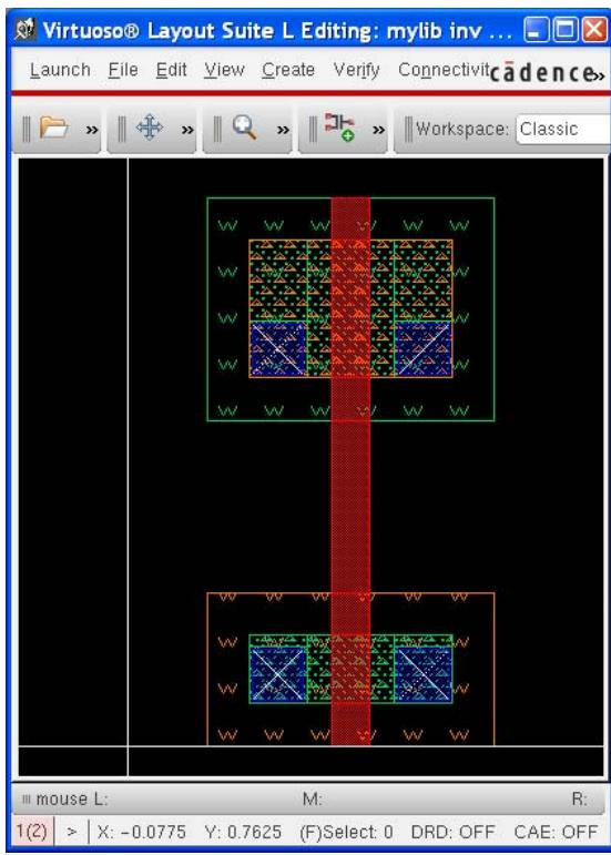
Another type of shape that you can create is a paths. Connect the drain nodes of the NMOS and PMOS transistor as follows:
