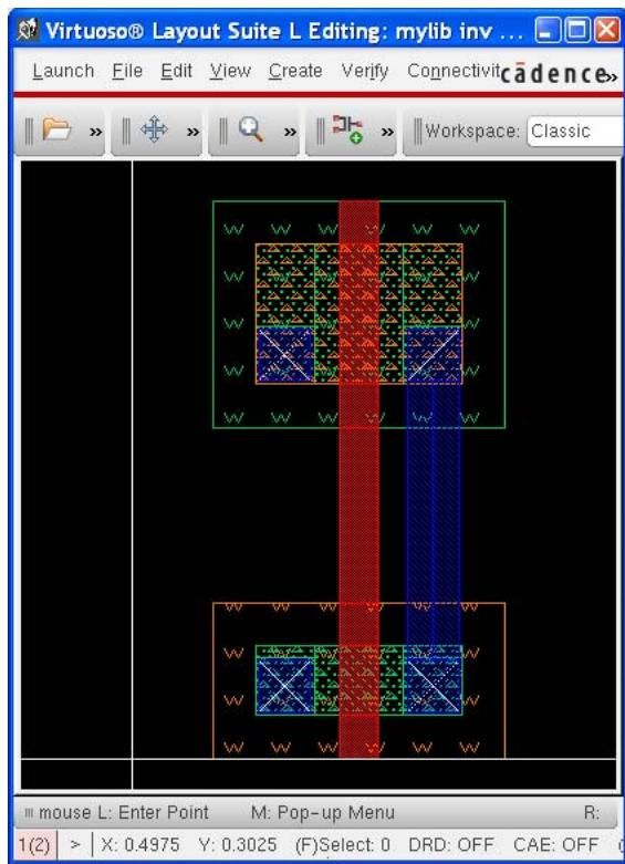
If you don't like the way your drawing turned out, you can select a shape and delete it with the delete key, or you can hit "s" (for stretch), and click on one of the sides of a path or rectangle to stretch it into the position that you like.
