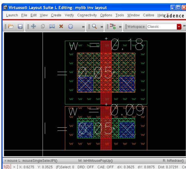
you should be able to figure out that the NMOS uses the following layers: **pwell**, **active**, **nimplant**, **poly**, **metal1**, **contact**, and **text**. The PMOS is like it, except that it uses layers **pimplant** and **nwell** instead of pwell and nimplant.
