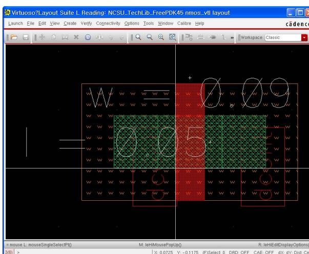
Draw NMOS and PMOS transistor. Finally the transistor looks like this.
