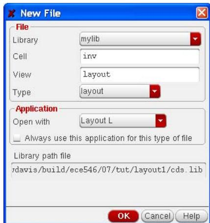
Alternatively, you can select the "Layout L" tool, instead of typing out the view name. This will automatically set the view name to "layout".
