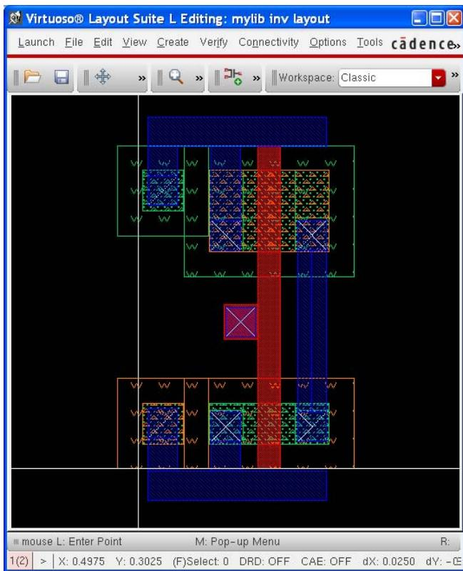
All of the **Metal.4** rules should be passing, now, except for the POLY via that we just created. To fix this error, extend the **metal1** shape to the left of the contact by 65nm, as shown below. That will fix the error.
