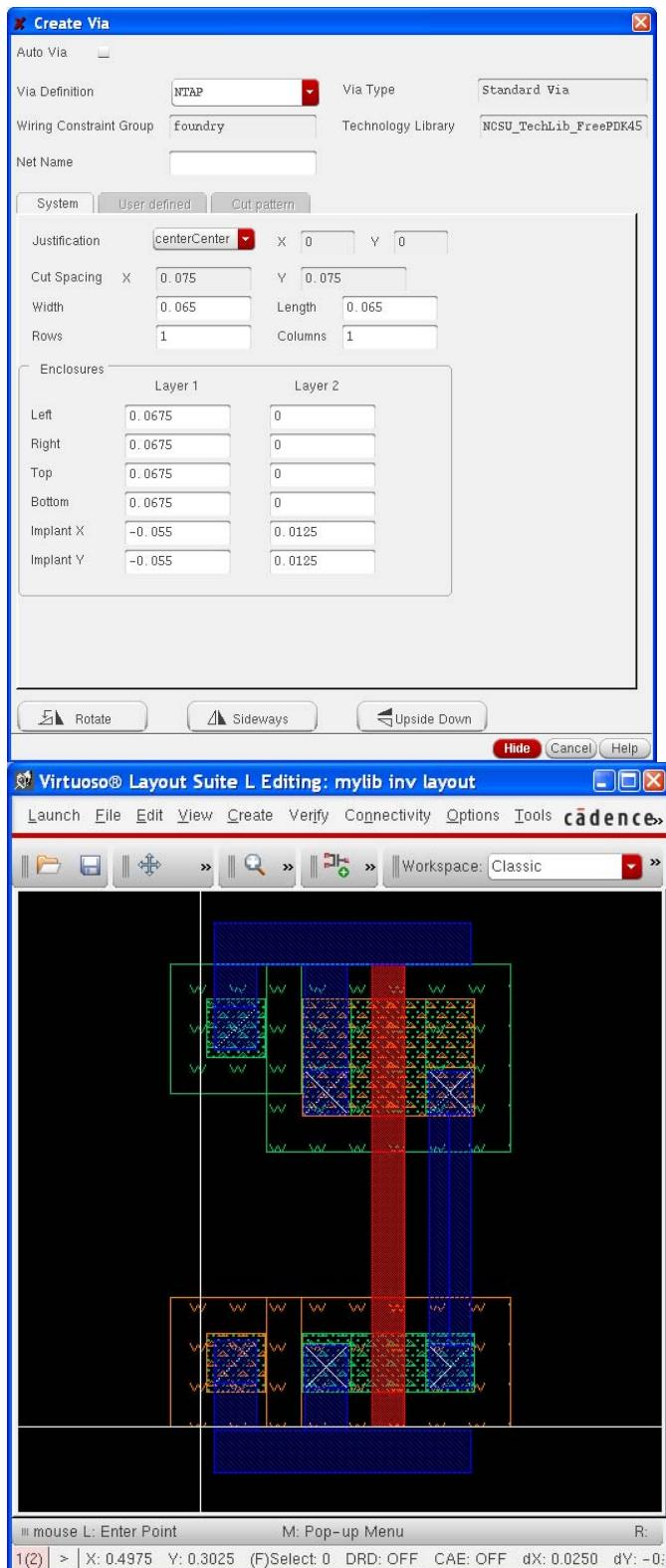
Next, add a gate-connection in *metal1*, with a *metal1-to-poly* via. Do this by choosing **Create->Via...** again and set the contact type to **M1\_POLY**. Position the via as shown below.
