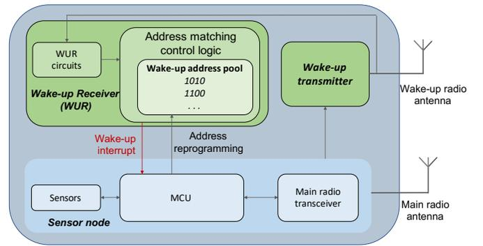
Fig. 2: The architecture of a wake-up radio-capable device.
