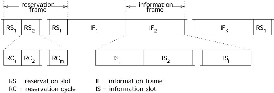
Figure 6.11 Frame and slot structure of FPRP.
