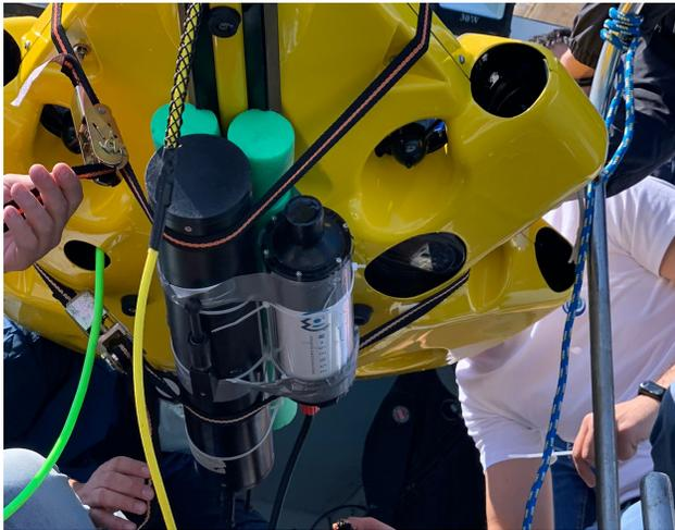
Fig. 3. The Zeno AUV with the WSENSE acoustic modem.
