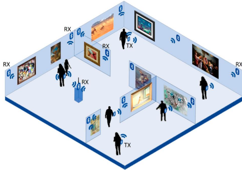
Fig. 2. Diagram of a LOS-based localization system for a museum. [9]
