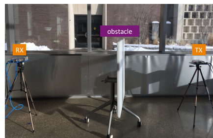
Figure 12: LOS blockage with a wooden table.
