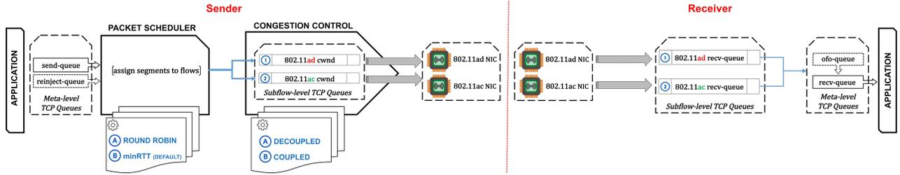
Figure 1: MPTCP Architecture (Sender and Receiver)
