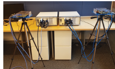
Figure 1: Two X60 nodes, each attached to a SiBeam phased array module.
