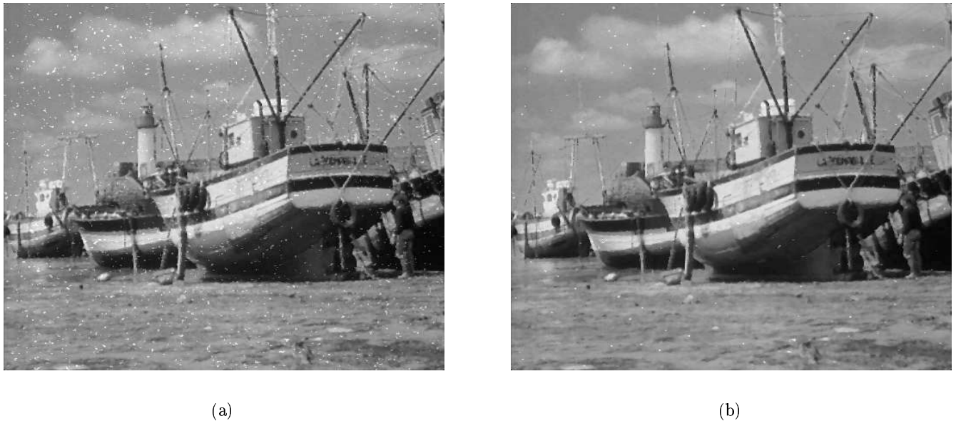
Fig. 8. Restored “boat” image by, (a) the 3 \times 3 median filter, PSNR = 25.0612 (dB), (b) an ATPMF implemented in rows, a = 1 , b = 1 , PSNR = 27.7221 (dB). Noise ratio is 20%. Noise has a uniform distribution between 0 and 80.
