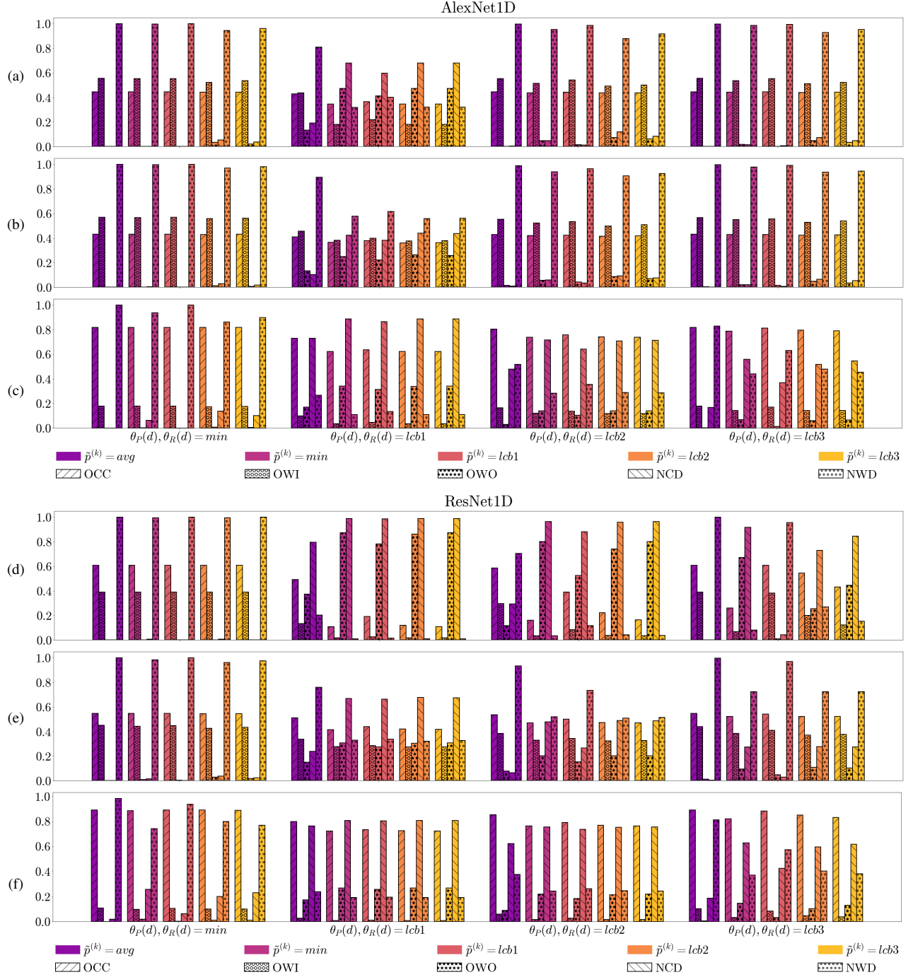
Fig. 5. Performance of AlexNet1D (a,b,c) and ResNet1D (d,e,f) models for different combinations of statistics used for thresholds \theta_P(d), \theta_R(d) and transmission prediction probability (TPP) \tilde{p}^{(k)} . Presented results are for datasets with |\mathcal{N}| = 500 in-library devices: WiFi dataset (raw transmissions (a,d) and their equalized versions (b,e), and ADS-B dataset (c,f). Models are evaluated on five metrics: OCC, OWI, and OWO for old device transmissions, and NCD and NWD for new device transmissions.
