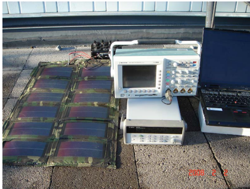
Fig. 11. Solar PV array outdoor test platform.
