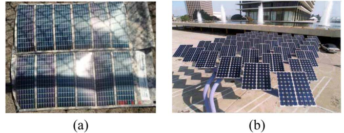
Fig. 1. Shadow configurations. (a) Shadow on portable solar array. (b) Shadow from one array cast on another array.
