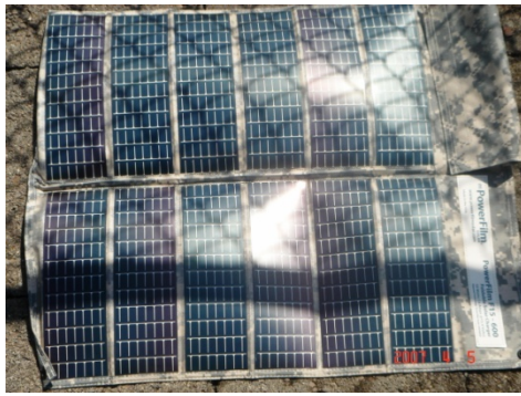
Fig. 1. Shadows on latest generation portable, flexible solar arrays
