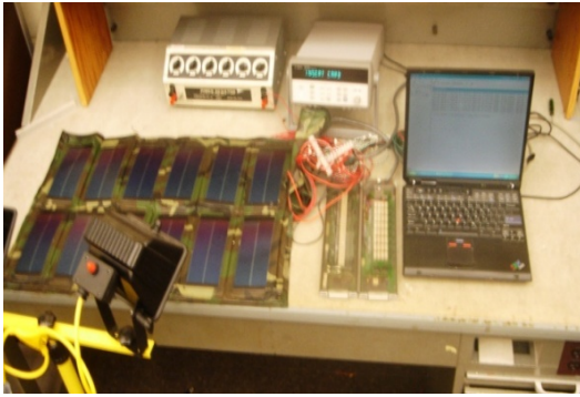
Fig. 8. Solar PV array indoor test platform
