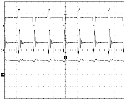
Fig. 13 Waveforms of Dual-Bridge DC-DC Converter with ZVS. V_{in} = 64V , V_o = 3.30V , i_o = 30A . From bottom trace to top trace: 1. i_L (25A/div) 2. V_s (5V/div) 3. V_{DS,D} (50V/div). Time base: 2ns/div
