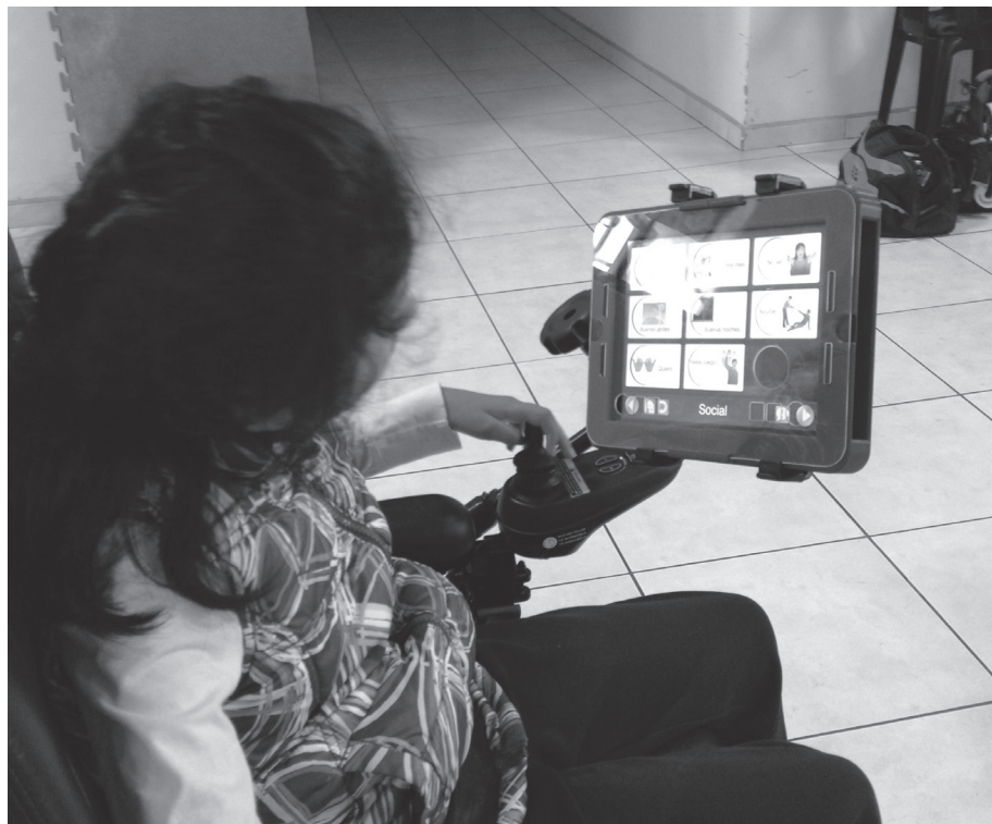
Figure 3. Alternative and Augmentative Communication System With iPad, Magic Arm, 3-Dimensional Printed Case, and Key Guard
