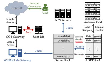
Figure 1: Arena access system diagram.
