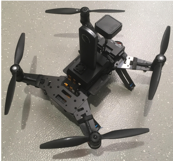
Fig. 1. Ricoh Theta S 360° camera mounted on Intel Aero drone
