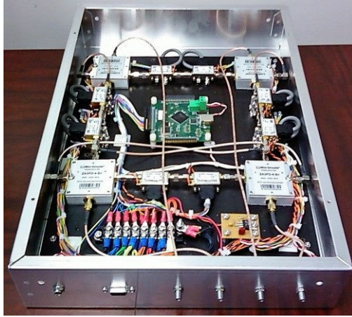
Figure 2. Network emulator, RFnest TM (4-node analog version).
