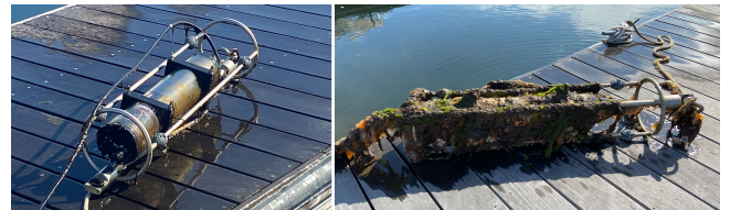
Figure 4: Images of the SDUM, that is deployed for 34 days, before (left) and after (right) biofouling.
