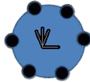
Fig. 1. A visual representation of a catom with a nanoantenna in its center.
