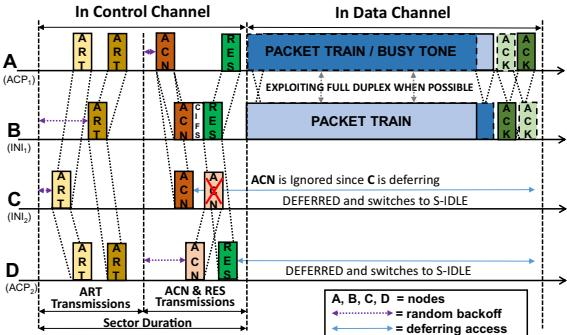
Fig. 3. Timing diagram of VL-MAC.
