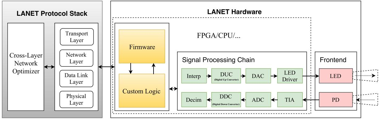
Fig. 2. Reference Architecture of LANET Node.
