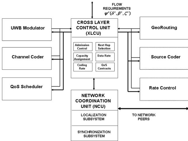
Fig. 1. Architecture of the cross-layer controller.
