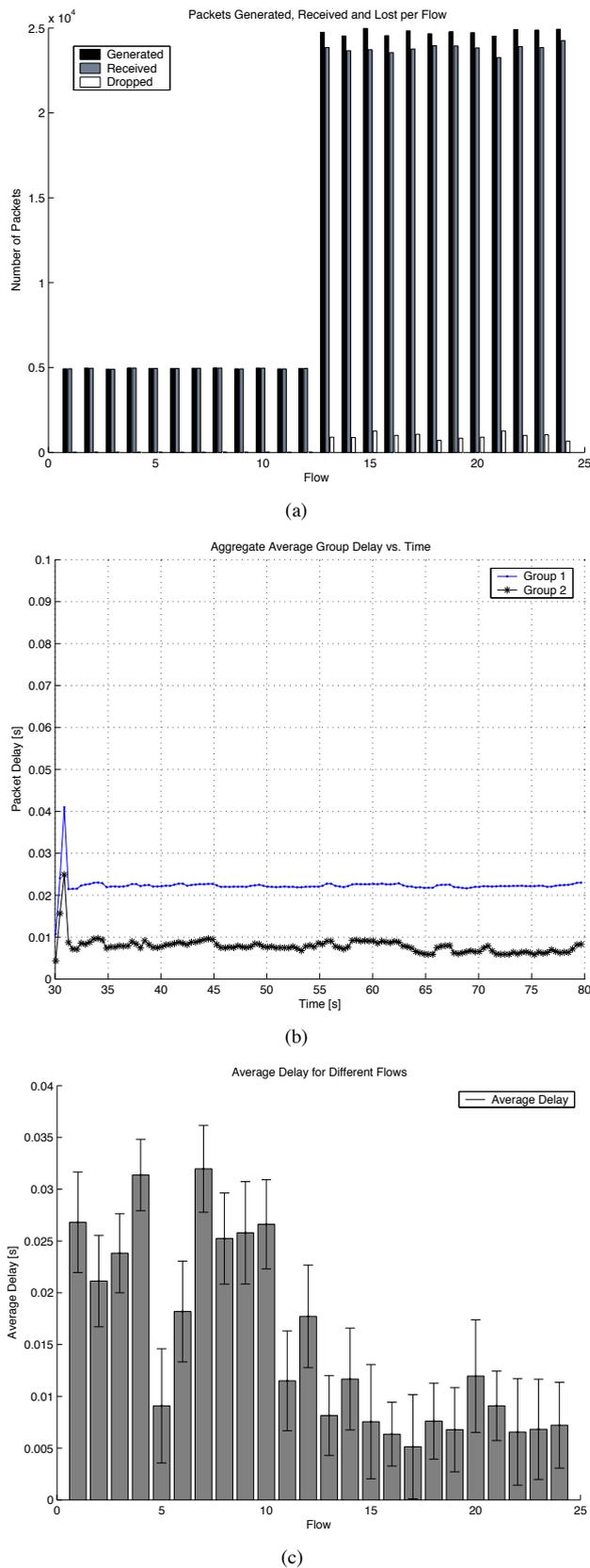
Fig. 5. Scenario 2. Packets Generated, Received and Lost per Flow (a) Aggregate Average Group Delay vs. Time (b) Average Delay for Different Flows (c).
