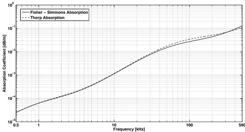
Figure 23.3 The Fisher and Simmons and Thorp’s absorption coefficient.
