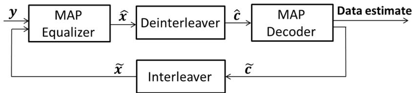
Figure 23.7 Receiver section with turbo equalization.
