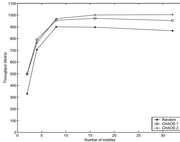
**Fig. 6.** FTP throughput vs. number of MSs varying matrix scanning methods.
