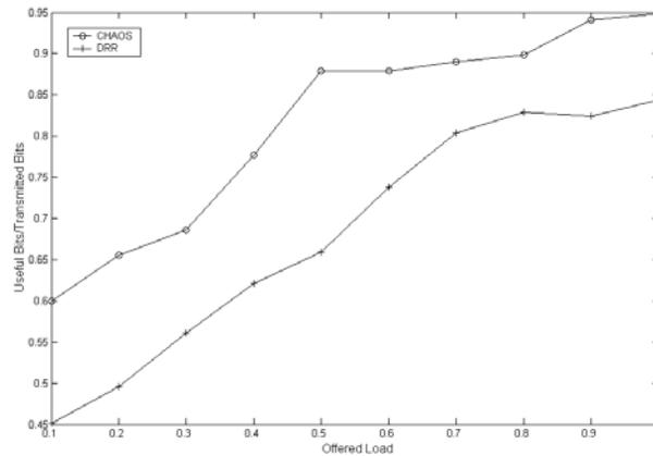
**Fig. 9.** Received Bits/Transmitted Bits vs Offered Load with different scheduling disciplines.
