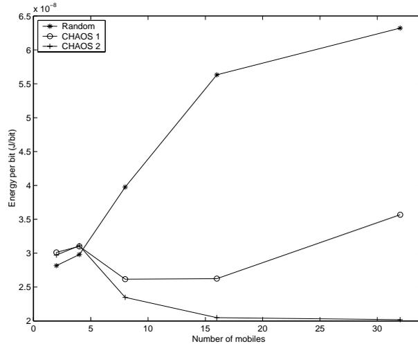
Fig. 7. Energy per bit vs. number of MSs varying matrix scanning methods.
