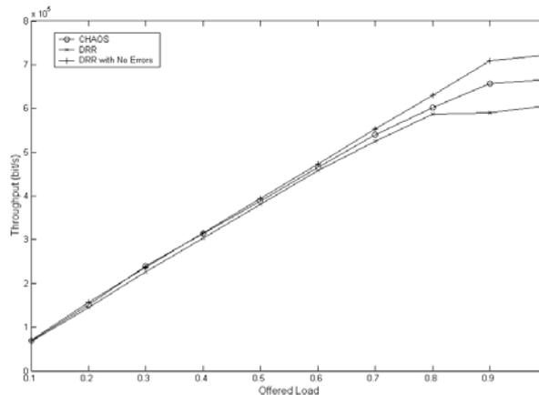
**Fig. 8.** Throughput vs Offered Load with different scheduling disciplines.
