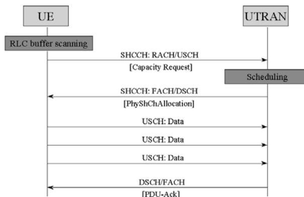
**Fig. 5.** USCH channel allocation procedure.
