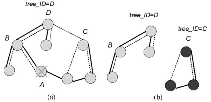
Fig. 4. Self-healing behavior when the network gets disconnected.
