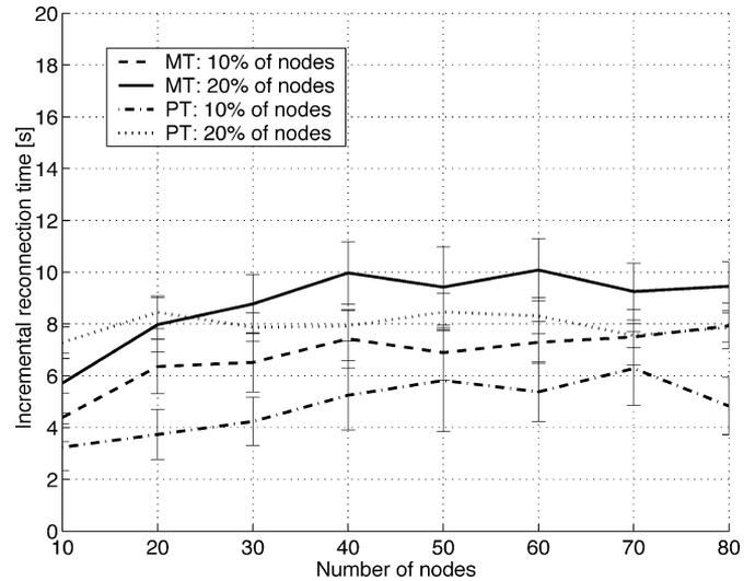
Fig. 10. Reconfiguration time in primitive and meshed topologies.
