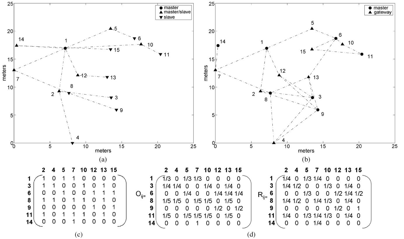
Fig. 15. Illustrative example. (a) Primitive topology. (b) Meshed optimized topology. (c) Matrix describing the optimized topology. (d) Matrices used to calculate the average normalized capacity.
