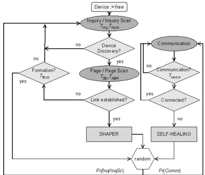
Fig. 2. Evolution of states for a Bluetooth device.
