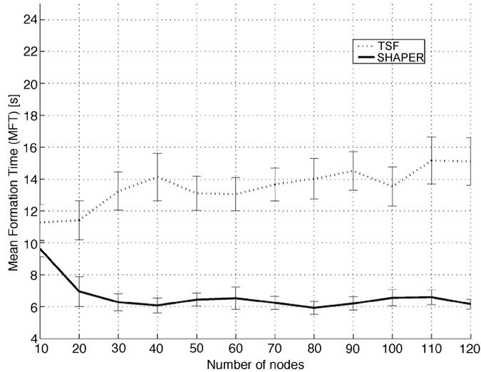
Fig. 6. Formation time: Performance comparison between TSF and SHAPER.
