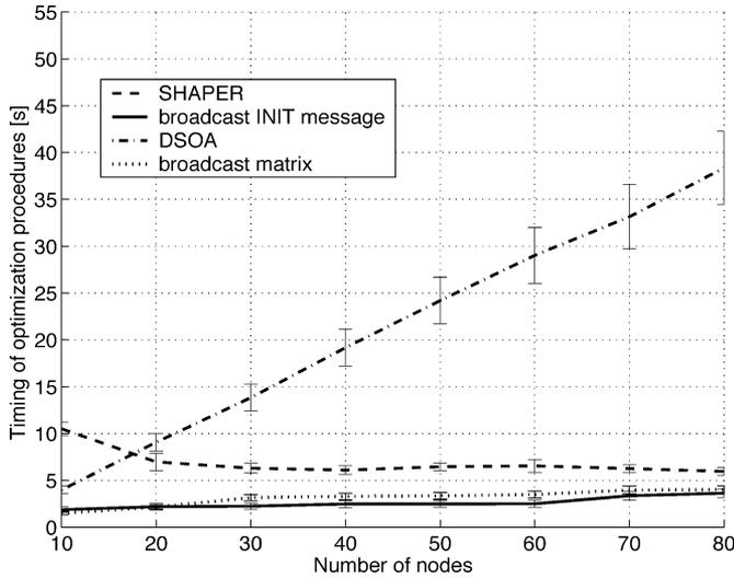
Fig. 12. Time needed by the SHAPER-OPT procedures.
