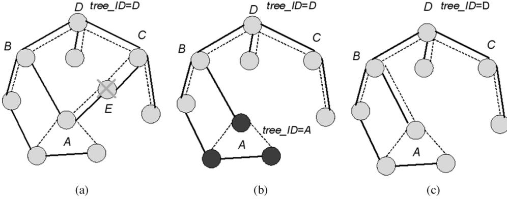
Fig. 5. Self-healing behavior when the network is still connected and two logical trees merge.
