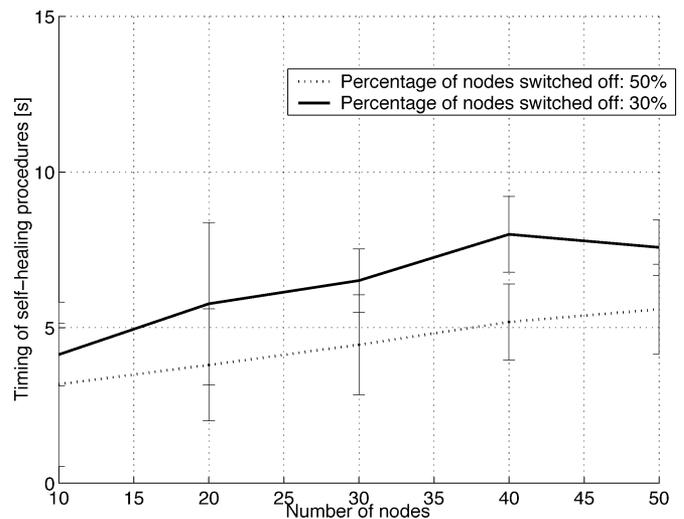
Fig. 11. Time needed for the self-healing procedures in meshed topologies.
