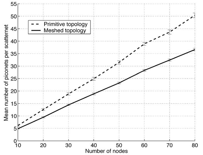
Fig. 13. Mean number of piconets for primitive and meshed topologies.
