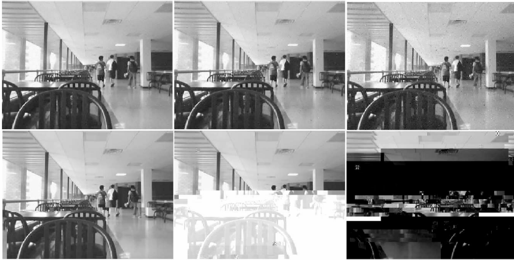
Fig. 2 Surveillance Image with CS (above) and JPEG (below) for BER (a) 10^{-5} (b) 10^{-4} (c) 10^{-3} .
