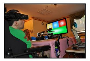
Lynxmotion SSC-32 servo controller, a GUI created through C# and XAML and ITU Gazetracker software. The M100RAK robotic arm kit gives four degrees of freedom, and is scaled to the size of an adult human arm. This allows the motions to be as natural and fluid as possible.The
